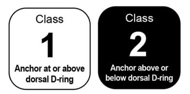
A. Visible "Class" icons must be provided on the SRL label to clearly identify the SRL Class.
